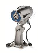
The integrated Fike Video Analytics software can detect an event up to 100 ft (30 m). Detected events are automatically recorded 24/7 and saved to the video server for post-event replay and download. Smoke detection is used only for well-lit, indoor areas and shall not be used in outdoor environments. By default, the smoke detection algorithm is disabled and must be enabled for use. Refer to the Robotic Fire Watch System manual for instructions.
